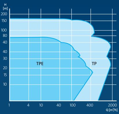
Grundfos TP/TPE is a comprehensive range of high efficiency In-line pumps. They feature the world-renowned Grundfos Blueflux® motor as standard and the TPE has an integrated frequency converter that ensures maximum efficiency at all times.
